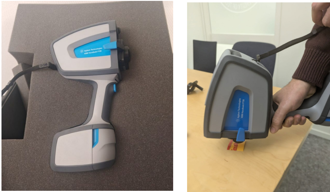
Figure 1 Left: Handheld FTIR Spectrometer; Right: Measurement process.
